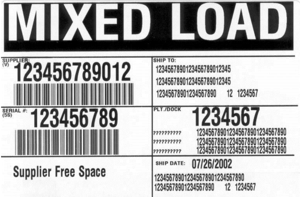
Figure 7: Mixed Load Label format
