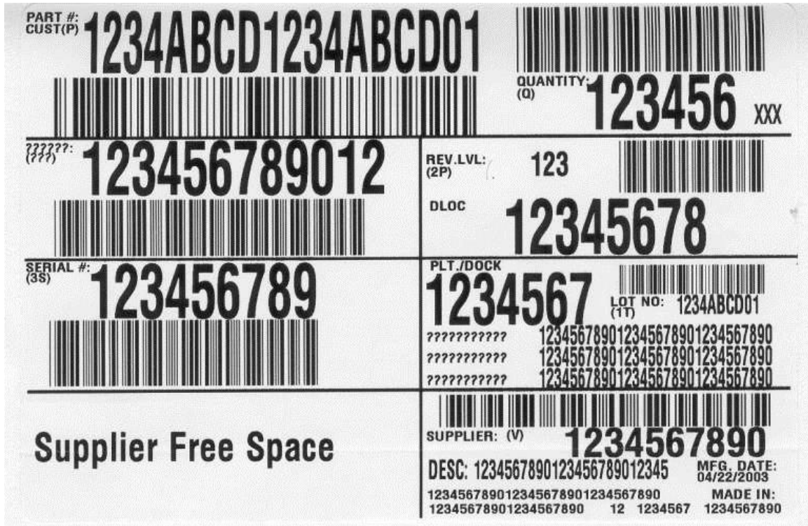
Figure 5 Container Label Standard Sample
